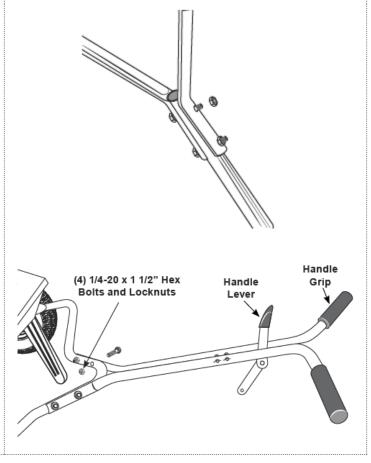
**Step 4:** Slide the ends of the Control Tube Braces over the Studs on the Shutoff Bar Brackets, secure with Cotter Pins. Install Hopper Handle on front of spreader using (2) 1/4-20 x 1/2" Hex Bolts and Locknuts.
