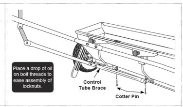
**Step 5:** To check spreader for completed shutoff, pull the Handle Lever back to the "OFF" position. Turn spreader over to see if the Shutoff Bar completely covers the holes in the bottom of the Hopper. If not, stand the spreader upright on Wheels push the Handle Lever forward to the "ON" position. Loosen the Bolts in the Hopper holding the Handle Brace. Push down on the Handle Brace and the front of the Hopper. Retighten Bolts and check the shutoff.
