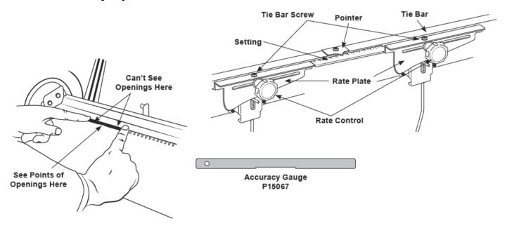
**Step 1:** Loosen both rate control knobs and set spreader setting at #4 1/2. With the operating lever in the open position, turn spreader upside down.
